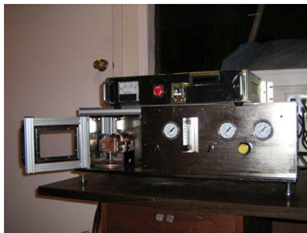
Fig. 7 Electron-optic unit of electro-thermoanalyzer ETA-100 (ALOFT, Berkeley, CA)
